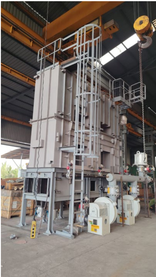
Picture 3 Three chamber, Anguil LoCarb-eRTO
